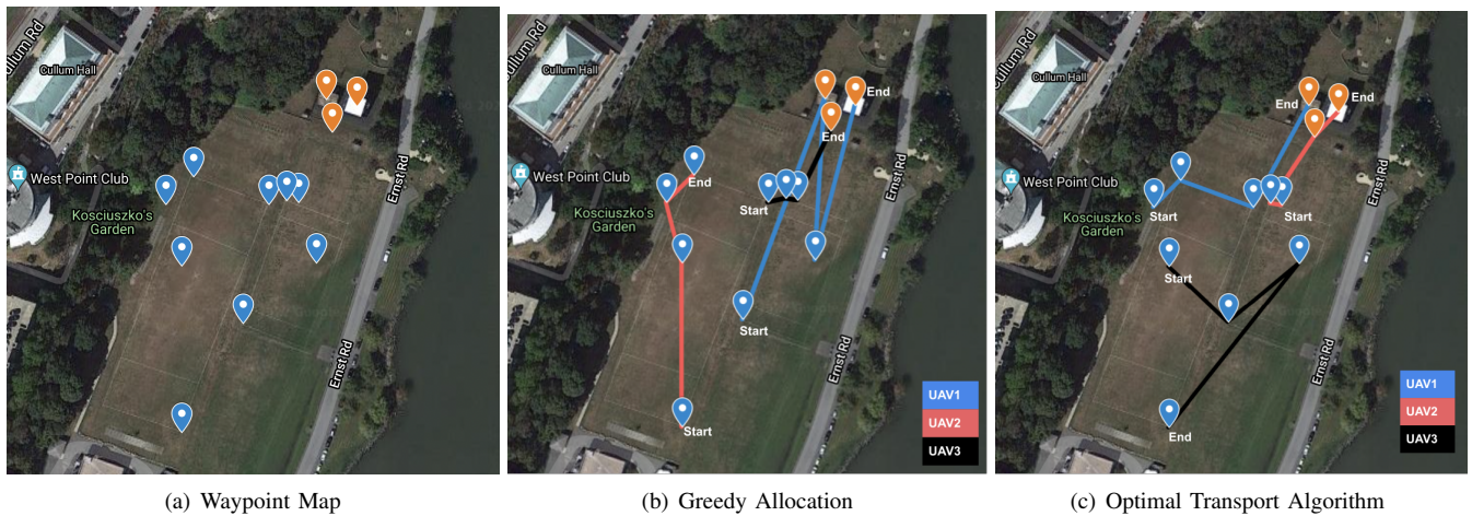
Fig. 4. (a) shows the location of the twelve waypoints, blue indicates a waypoint where there is no chemical present, orange indicates a waypoint with chemical, (b) shows the path of the UAVs with the greedy algorithm, (c) shows the path of the UAVs using Alg.2
